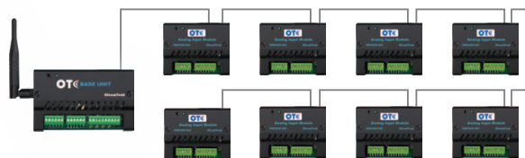
Typical installation of OleumTech expansion modules are mounted adjacent to the DH1 Base Unit on DIN rail in a NEMA 4 enclosure and connected with supplied inter-module connector cable. Expansion modules compatible for use only with DH1 Gateway.
