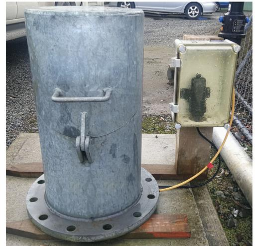
The LS1-P is a compact and configurable pressure based depth sensor. It provides a cost effective solution to wide scale monitoring of water levels in confined spaces. The LS1-P transmits accurate water level data directly to the Waterwatch Live cloud platform or integrated software.
