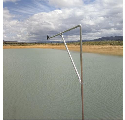
The LS1 is a highly configurable non contact water level sensor ideal for water storage and open waterway monitoring. Trusted by water utilities, city councils, regional governments and home owners around the world, the LS1 is proving to be the preferred solution for monitoring in remote areas.
