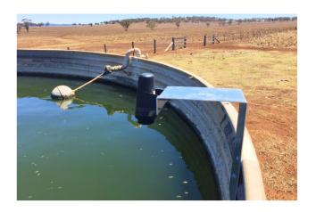
Waterwatch sensors are installed above tanks and troughs of any shape. Quick and easy installation is done with guided instructions on the Waterwatch mobile app. The hardwearing plastic enclosure is waterproof and UV resistant for long term deployment in harsh environments. With configurable measurement and transmission intervals, the Waterwatch sensor can be set up to suit your requirements.
